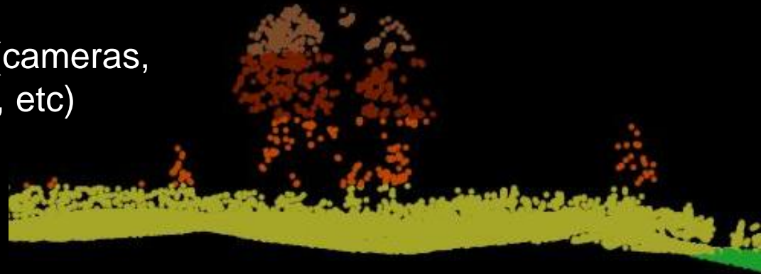
Point cloud profile from Lidar
