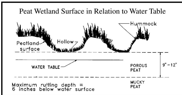
The water table (solid line) is near the bottom of the hollows (upper dotted line). Operations should stop when ruts reach 6 inches below the water table or 6 inches below the bottom of the hollows, whichever is lower. Peat is usually still porous 9 inches below the hollows, and ruts will heal in 2 to 3 years. Deep ruts (more than 12 inches below the hollows) will bring up well-decomposed, mucky peat and may take more than 20 years to heal.
