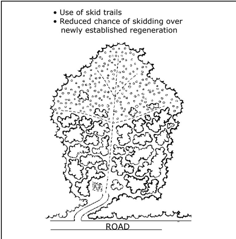
✓ **Plan a progressive harvesting technique** that avoids trafficking over pre-cut areas where possible. See Figure TH-2. For example, back-to-front harvesting techniques in frozen and unfrozen conditions can reduce site impacts during harvesting. Advantages of this method include the following:
