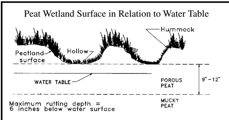
**Figure TH-10:** The water table (solid line) is near the bottom of the hollows (upper dotted line). Operations should stop when ruts reach 6 inches below the water table or 6 inches below the bottom of the hollows, whichever is lower. Peat is usually still porous 9 inches below the hollows, and ruts will heal in 2 to 3 years. Deep ruts (more than 12 inches below the hollows) will bring up well-decomposed, mucky peat and may take more than 20 years to heal.
