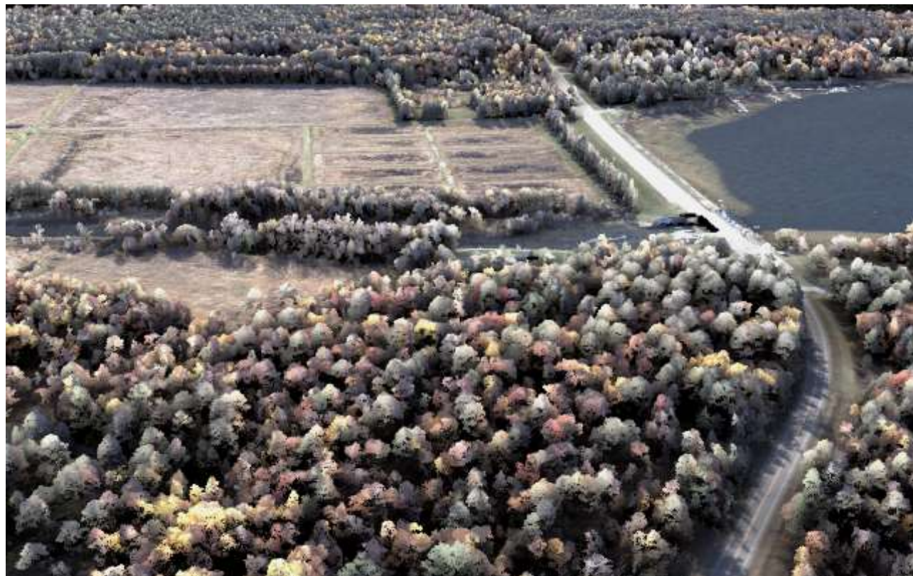
High Density Lidar Point Cloud Colorized by Photo During Peak Fall Color
