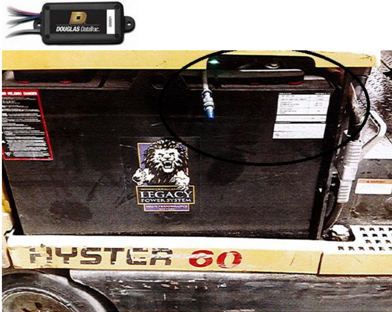
Figure 4. Battery Monitoring Device and Embedded Test Assembly
