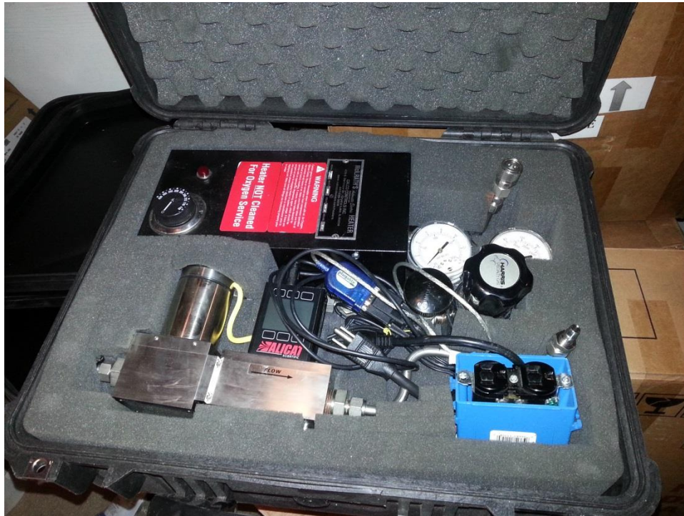
Figure 52: UC Davis tracer gas injection system with heated regulator, heater, and mass flow controller
