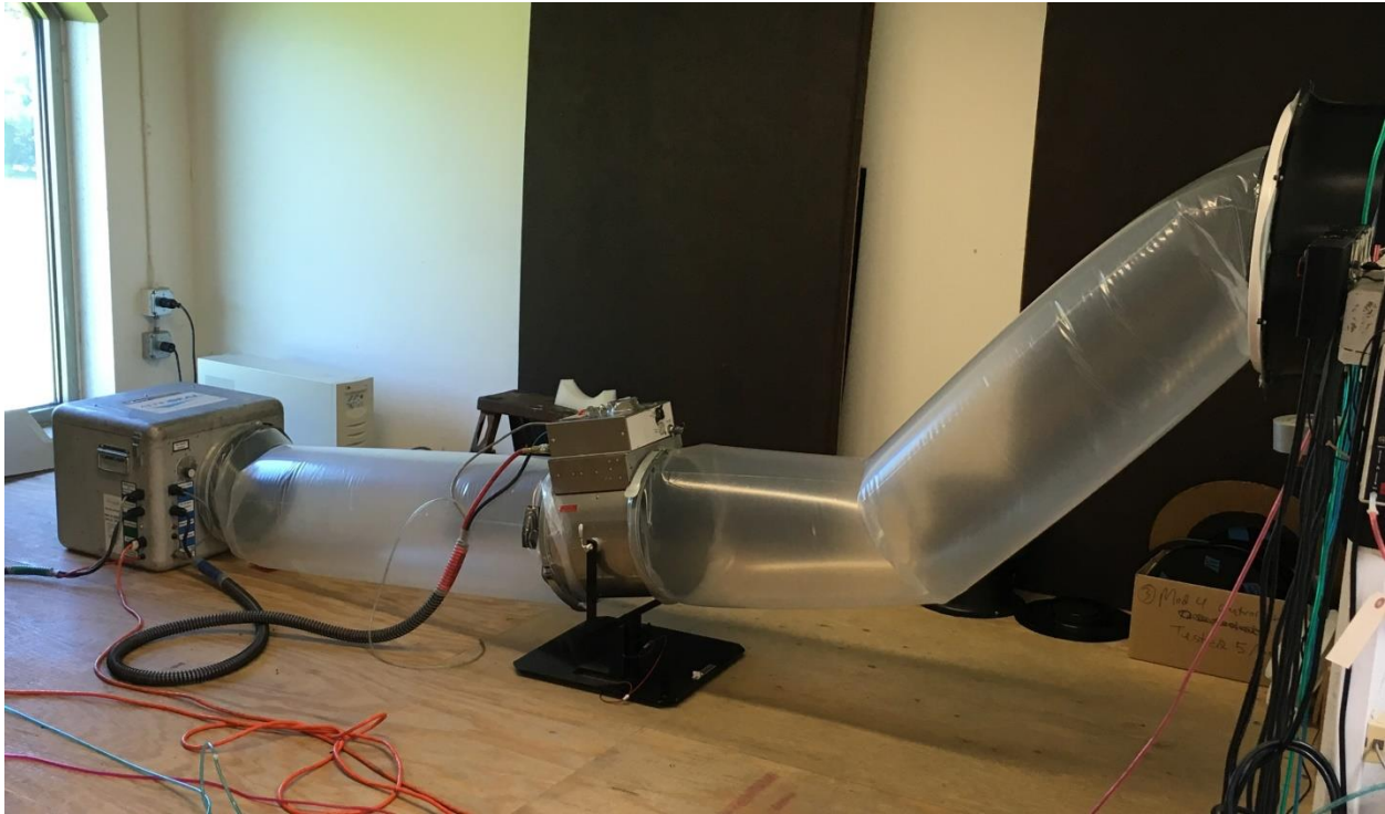
Figure 63: Complete testing setup (absent injection wand).
