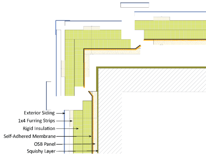
Figure 23 - Outside Corner Connection – Blind, Option 2 - Plan View
