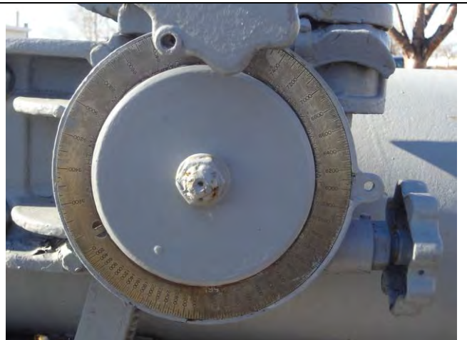
The vernier elevation scale, PL side of the gun. The brass was cleaned and coated in 2006 and remains legible.
