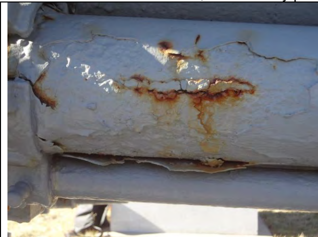
Corrosion breakthrough and paint failure, staining on PL recoil tube.
