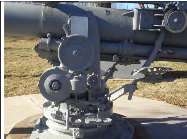
PL side showing trainer's seat, elevation wheels and other components.
