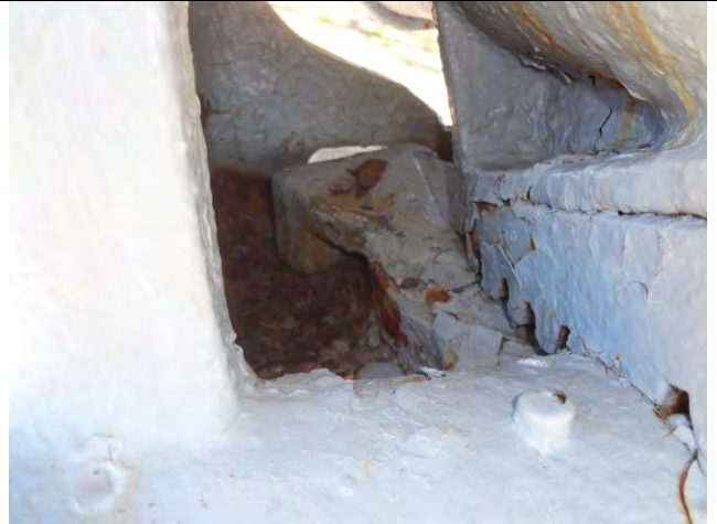
Overview of debris and rust accumulation 'inside' swivel support mount assembly below the recoil tubes and barrel
