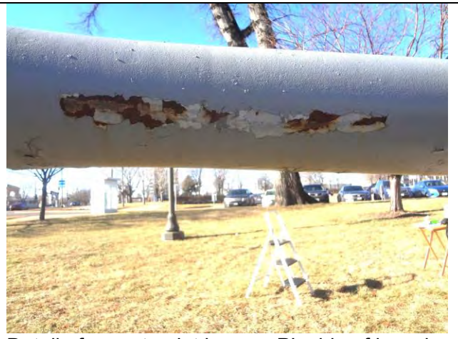
Detail of recent paint loss on PL side of barrel towards muzzle end.
