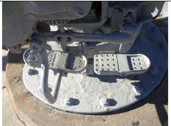
PL side foot rests. Painted brass. The foot rests on the PR side are also painted brass.
