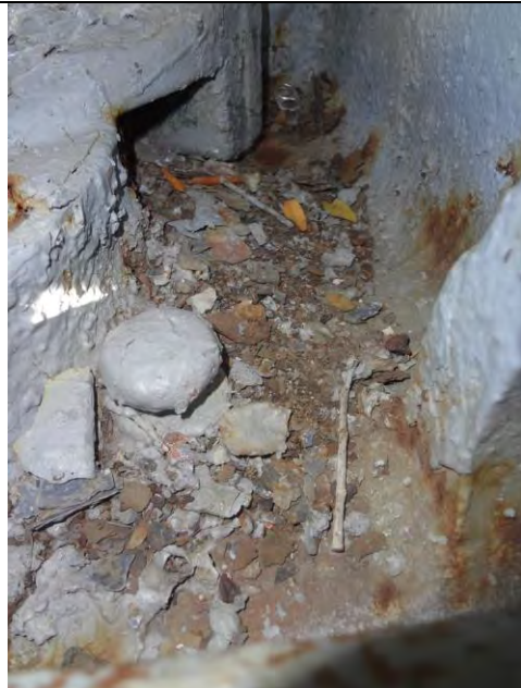
Detail of paint and rusted metal flakes on bottom of 'interior' of the swivel mount, PR side.
