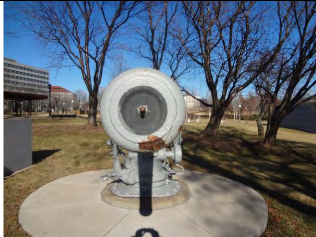
Overview of muzzle showing modified plumbing plug, installed in 2006.
