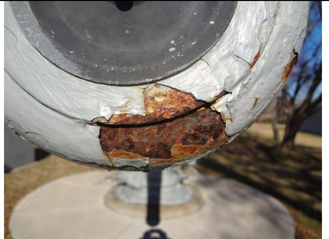
Detail of corrosion breakthrough and paint loss on lower margin of the muzzle rim.
