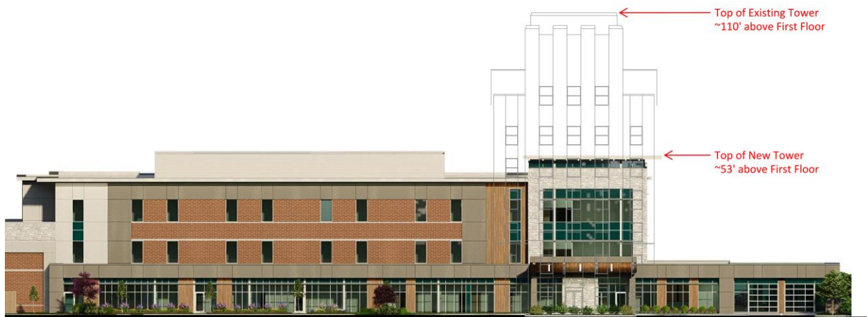
East Building Elevation with 1931 Original Hospital Tower Overlay (view from North Capitol Boulevard)
