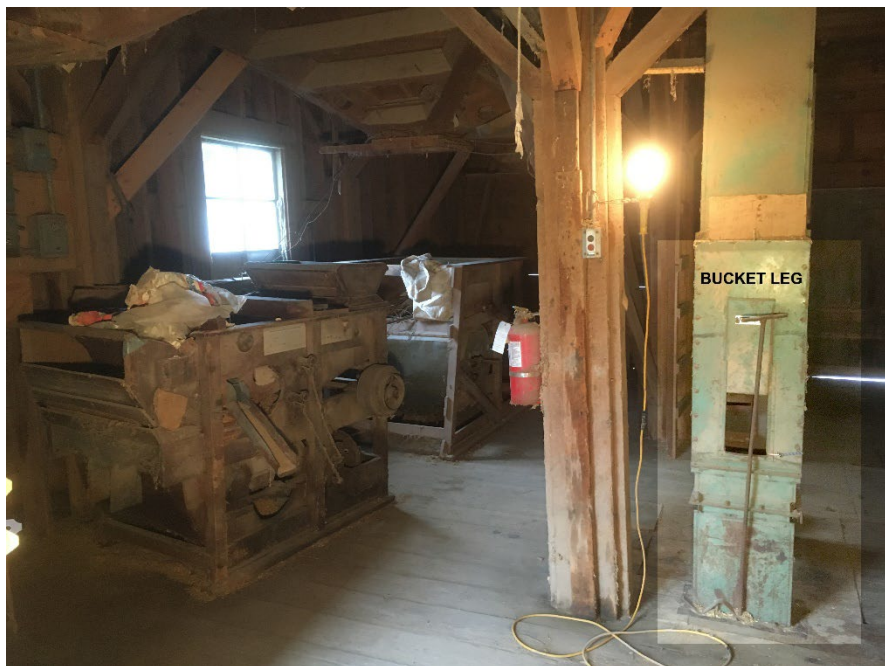
Photo #10 (MN_Fillmore County_Mc Michael Grain Elevator_00010) Interior view of leg, working house floor.
