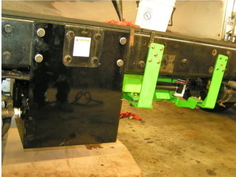
Figure 3. New Oil Tank
