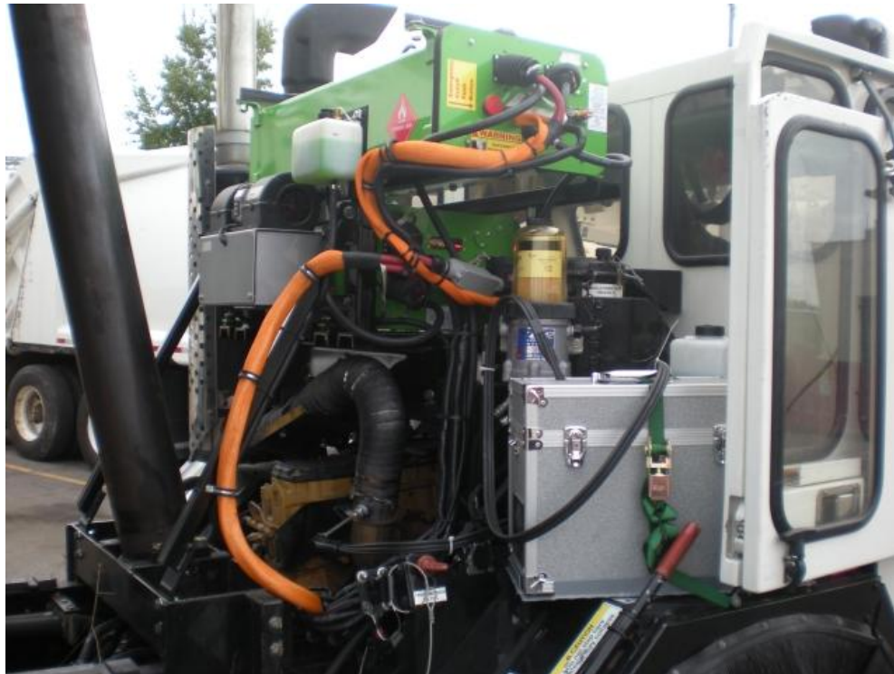
Figure 5. Greenline Emissions Sampler Mounted on Truck
